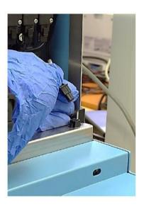
Remove two screws which hold pump in place, remove pump from the noise dumping foam.
