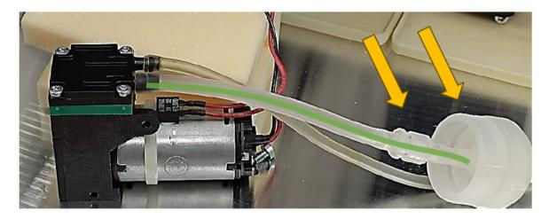
Assemble everything in reverse order. Place tubes and cables in correct locations. Make sure that grounding wire (left screw of pump's cover) is installed. Put all covers back.
