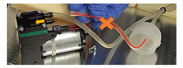
Install new tube (highlighted in green). Make sure that Luer connector is located next to the inline filter.
