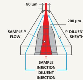
Patented hydrofocus flow cell and improved injector technology employs a diluent sheath to drive and maintain sample flow across the cuvette through the detection area while reducing cellular damage.
